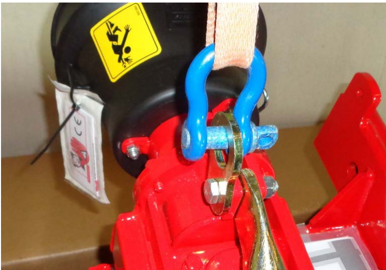
Figure 5 lift point on power harrow
