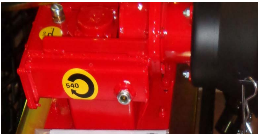
Figure 11 top gearbox with vent and sight-glass window
