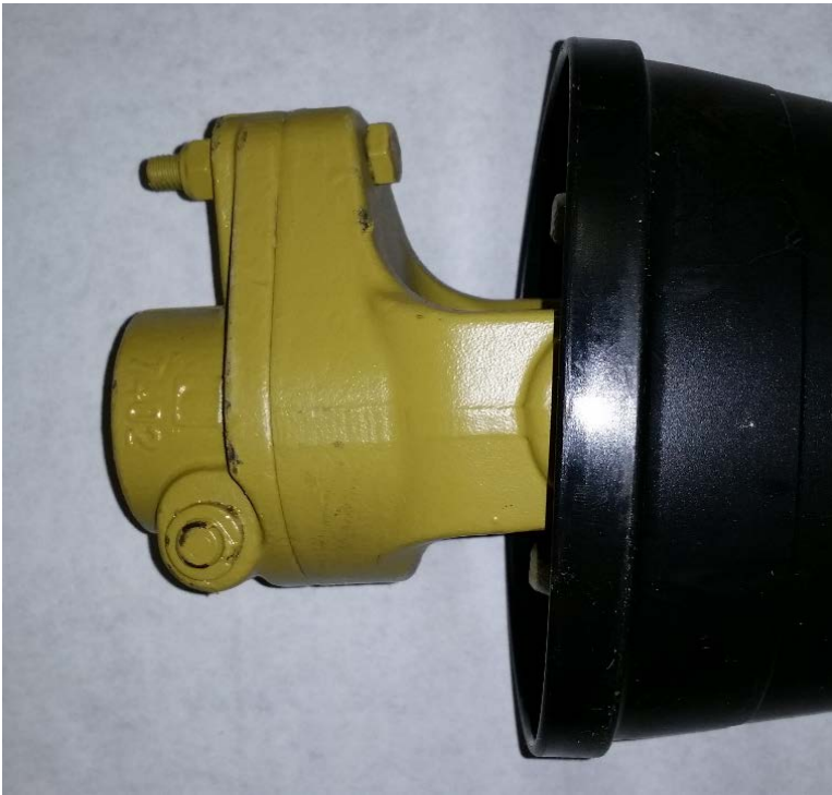
Figure 8 driveline with shear bolt
