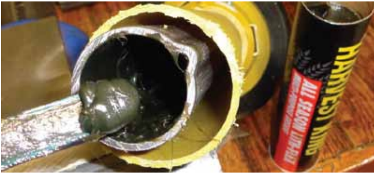
Figure 14 spread grease in outer shaft
