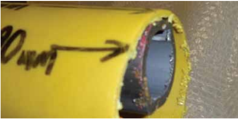
Figure 6 align end of tube to end of shaft
