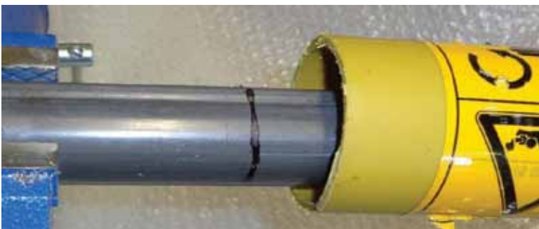
Figure 8 shaft is marked to cut off same length as plastic tube
