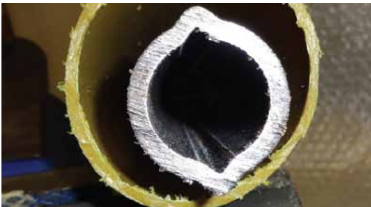
Figure 11 burrs and shavings must be removed
