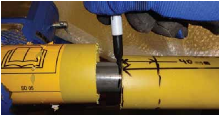
Figure 7 use tube to mark the cut length to steel shaft
