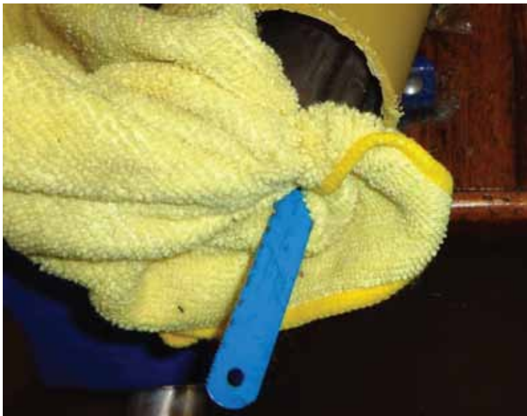
Figure 13 push towel into and around shaft to remove shavings
