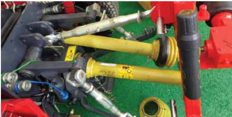
Figure 2 PTO shaft ends installed to mark overlap
