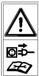
it is forbidden to carry out any maintenance work or to renew parts on the machine when it is running.
