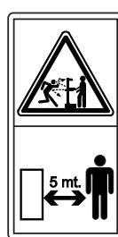
it is forbidden to stand in the range of action of the machine. apart from the operator, no other person or animal may be present within a radius of 5 metres from the machine.
