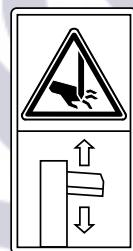
Danger of cutting or crushing of the hand: never touch hazardous areas while the wedge is moving.
