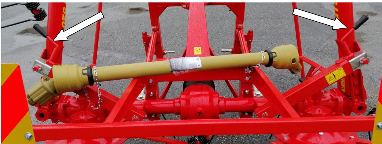
Manual locking device for arms lowering (lever)
