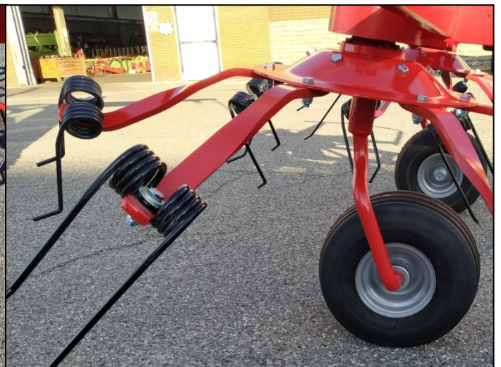
Twisted arms with hooked tines
