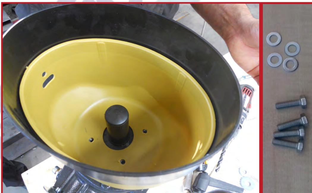
**42.** Take the PTO guard, position it on the gearbox and insert the washers and the screws.
