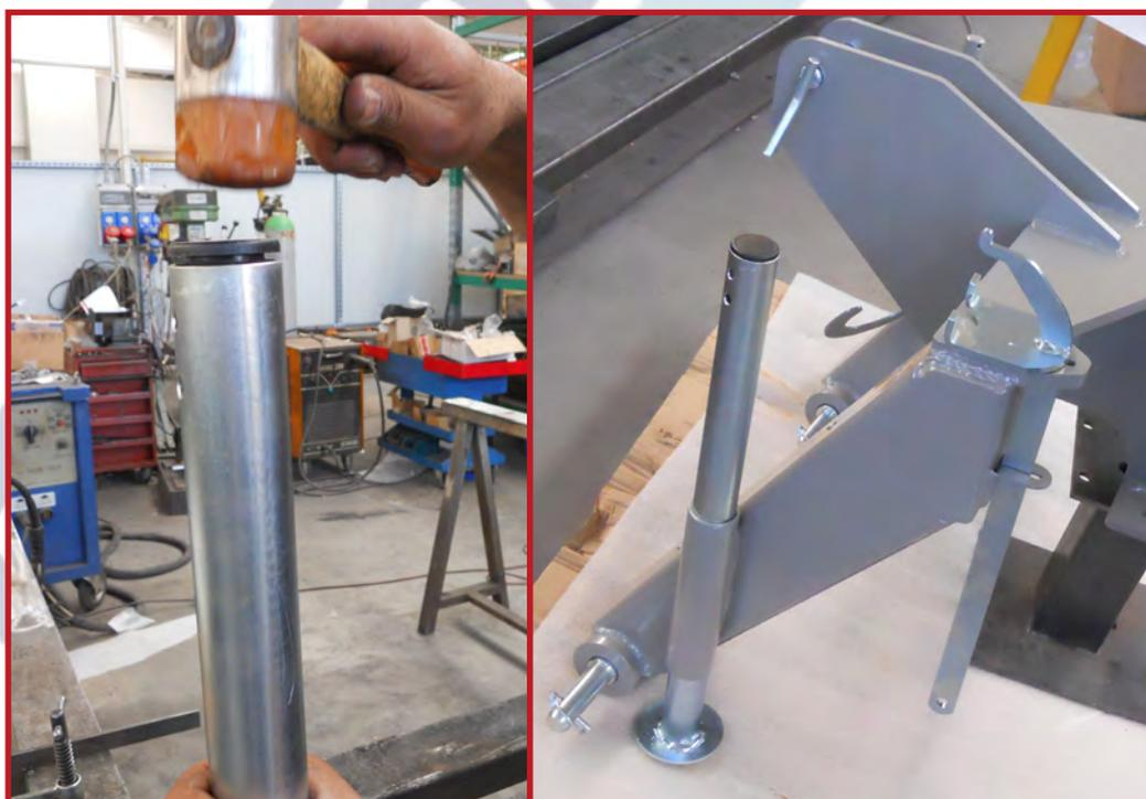
**34.** Take the foot and insert the plastic cap; position the foot in the 3rd point.
