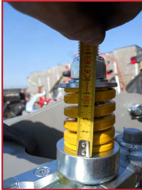
**81.** Regulate the spring tension (max. compression= 5,5 cm)
