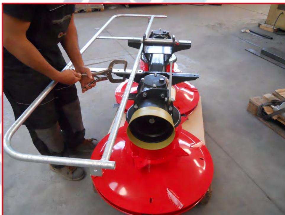
6. Lock the front frame guard on the cutter bar like shown in the picture.
