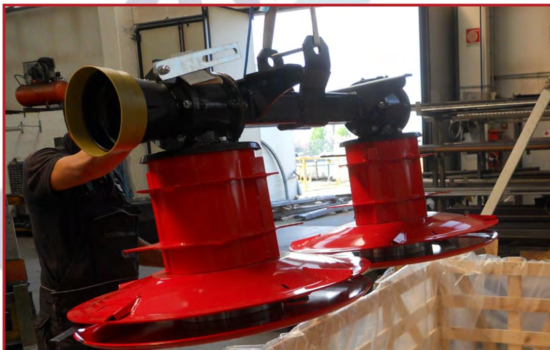
2. Remove from the wooden crate the cutter bar group and lay it on a stable surface.
