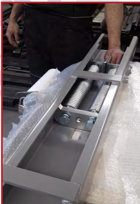
**54.** Insert the spring assembly in the upper "C" plate like shown in the photo.
