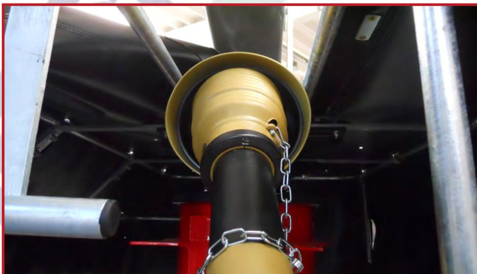
**72.** Take the intermediate PTO shaft and attach it to the machine.
