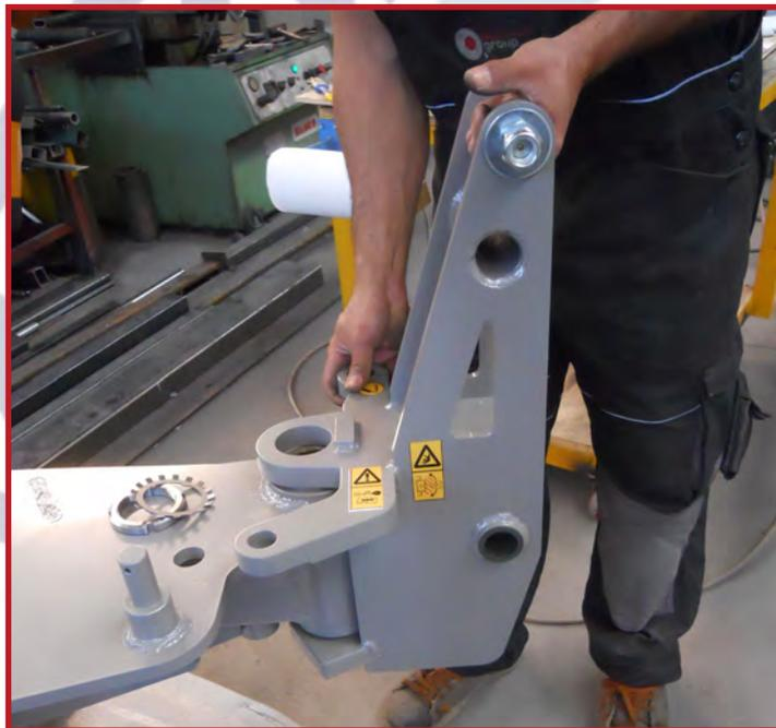
**28.** Position the pivoting assembly on the frame of the 3rd point like shown in the picture.
