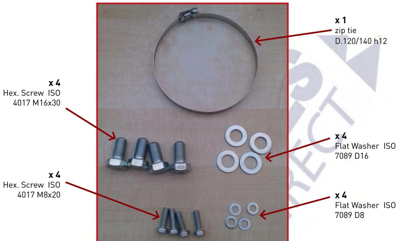
**41.** Screws necessary for gearbox's assembly.
