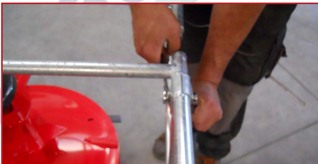
**14.** Tighten the locking of the guards pipe.
