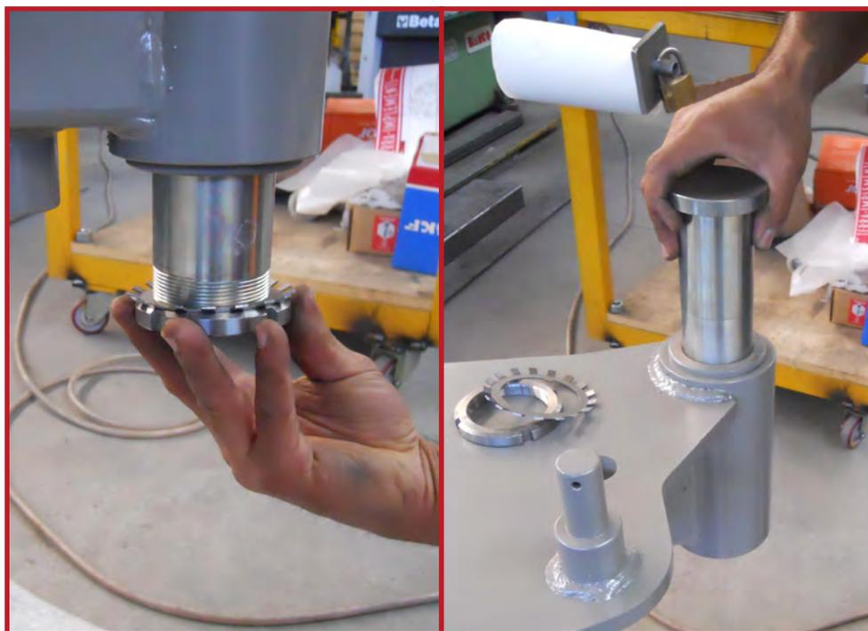
**25.** Remove the safety washer and the ring nut for extract the pin.
