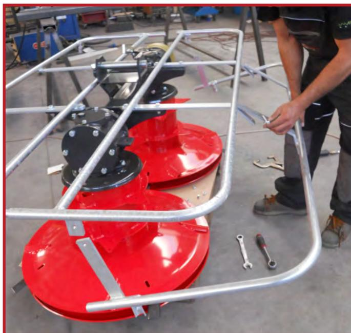
9. Take the extension front frame guard and fix it to the front frame guard like shown in the picture.
