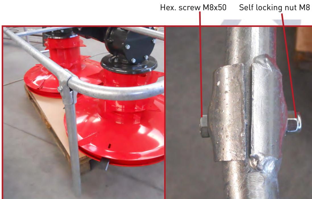
**13.** Take the guards pipe and fix them to the side of the protections with screws and nuts.
