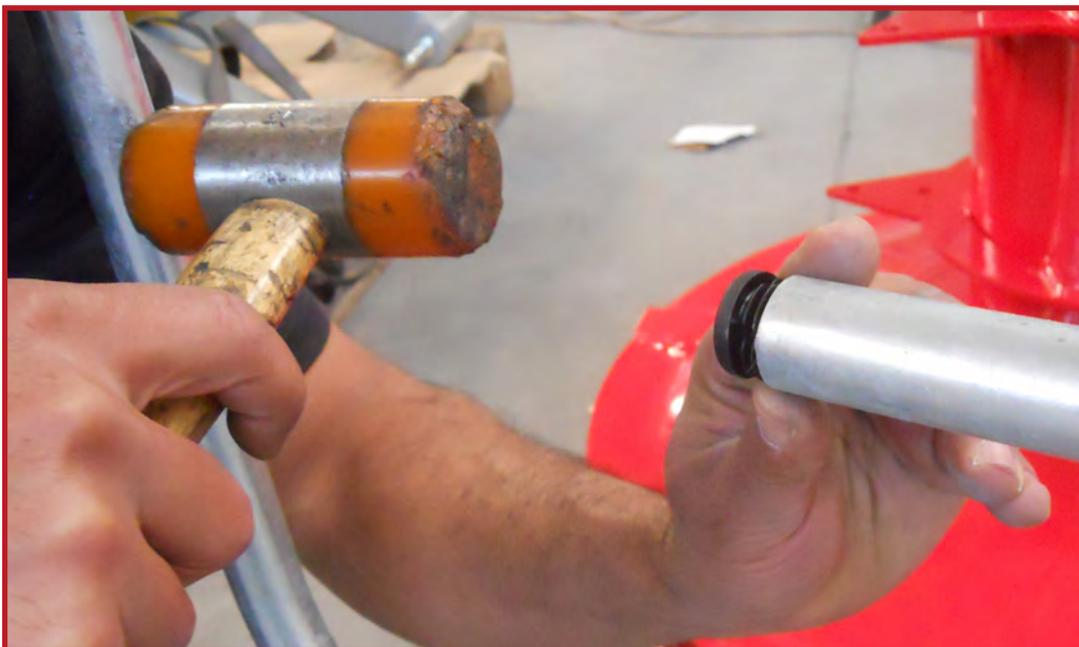
5. Take the front frame guard from the wooden crate and insert the plastic cap at the end of the tube like shown in the picture.
