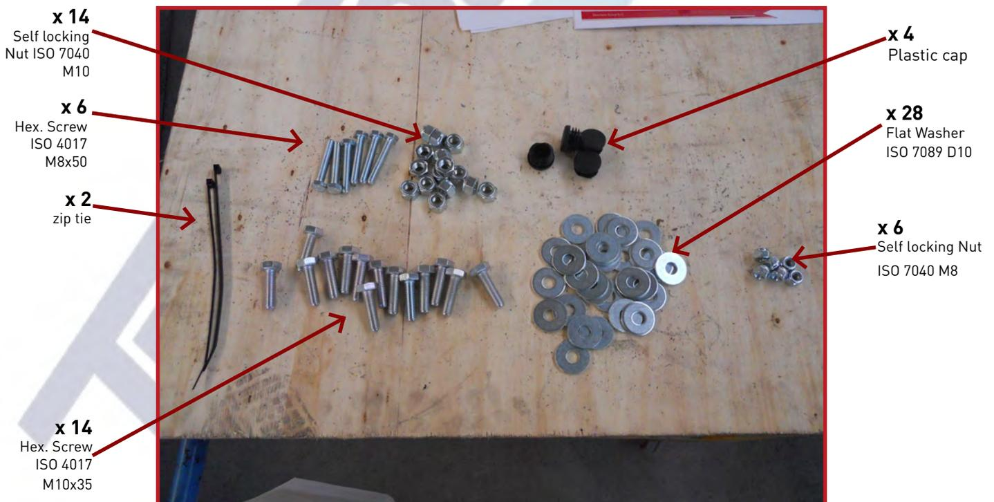
**4.** Screws necessary for the protection's assembly.
