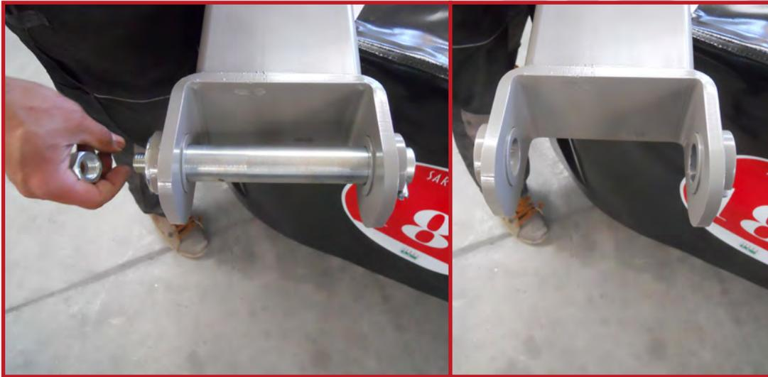
**47.** Remove the pin from the support beam.
