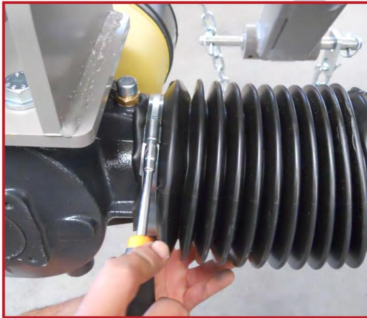
**75.** Insert around the rubber bellows the zip tie and lock it.
