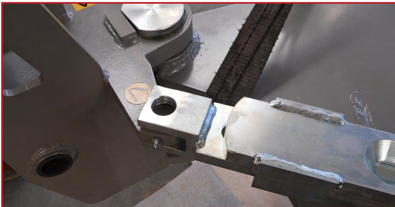
**37.** Position the end of the breakaway on the hole of the pivoting assembly like shown in the picture.
