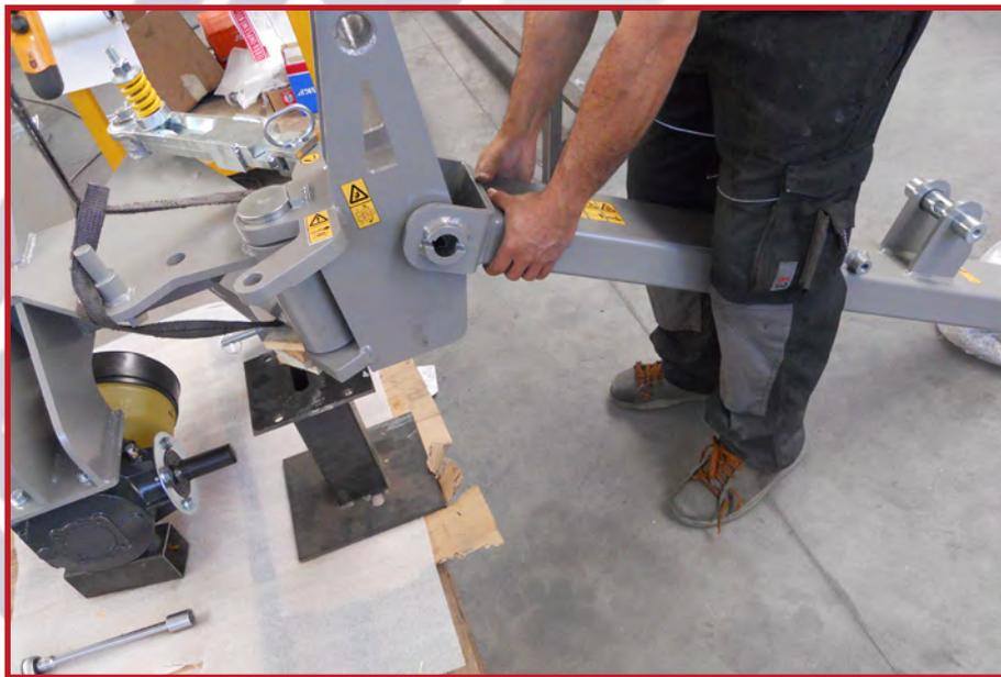
**48.** Position the support beam near the pivoting assembly by matching the holes.
