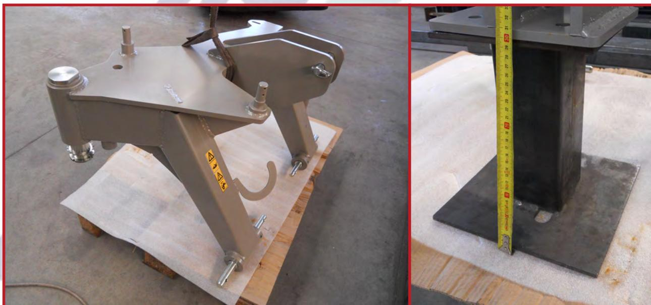
22. Raise the 3 point hitch and lay it on a support **high 30 cm** like shown in the picture.
