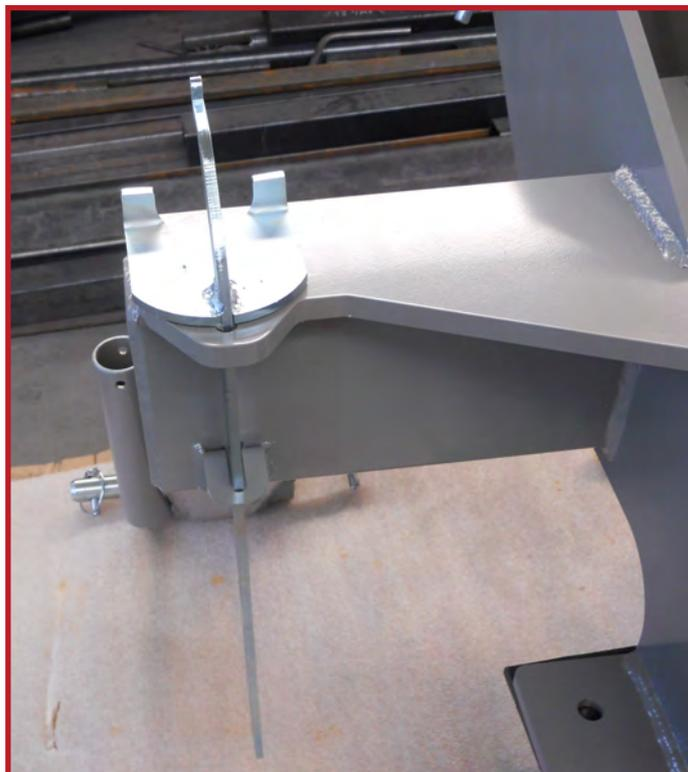
**33.** Insert the tool to release the blades like shown in the picture.
