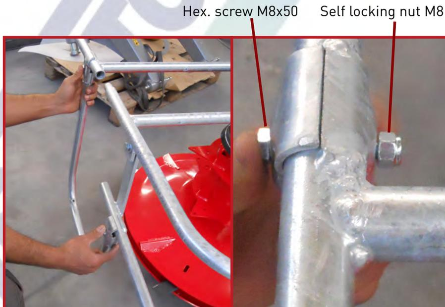
**12.** Take the U tube and fix them to the side of the guards with screws and nuts.
