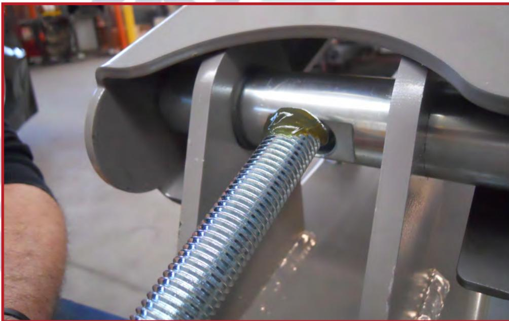
**60.** Insert the threaded bar in the hole adding some grease.
