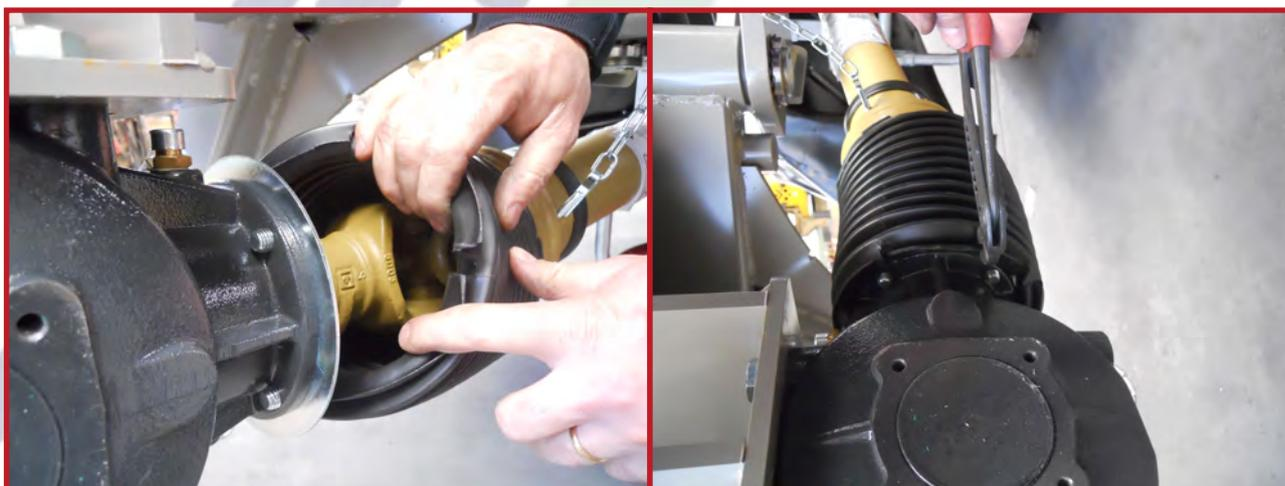
**74.** Attach the PTO shaft at the side of the gearbox and to overlap it to the circular plate.
