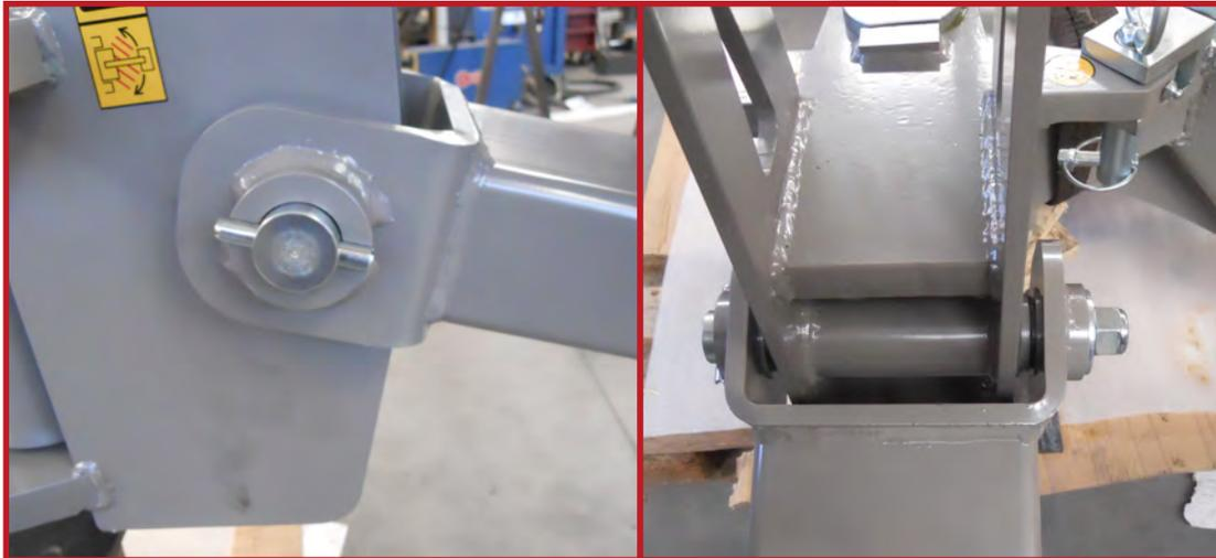
**49.** Reinsert the pin in the support beam and tighten the locking.
