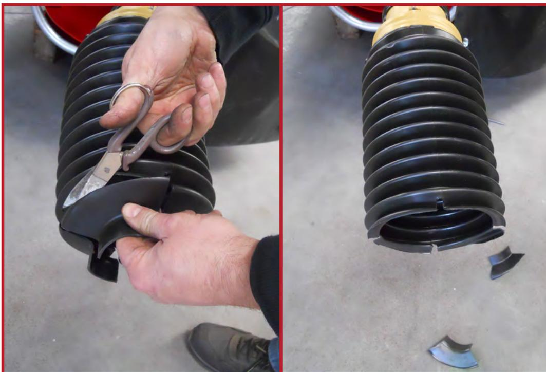
**73.** Cut like shown in the picture the rubber bellows.
