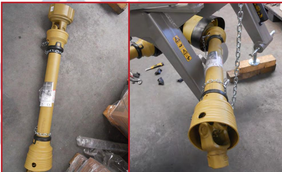
**78.** Take the other PTO shaft and attach to the gearbox.
