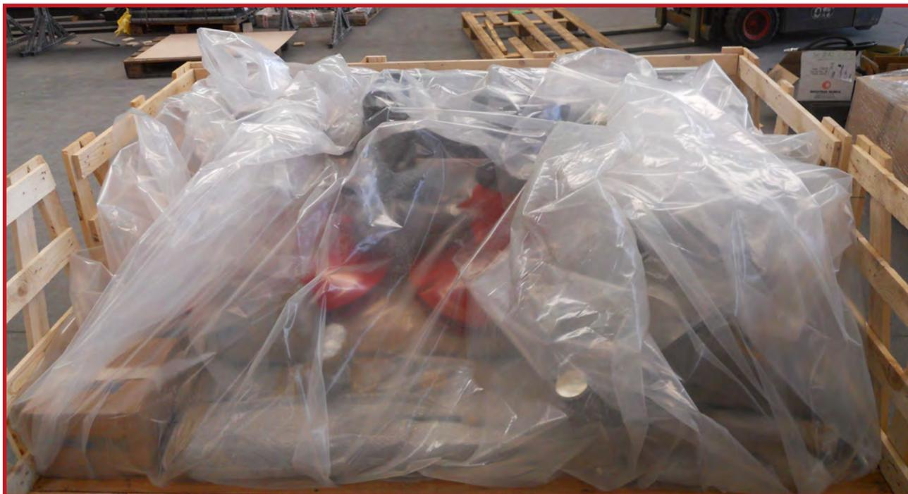
1. Remove the top from the wooden crate and cut the cellophane.
