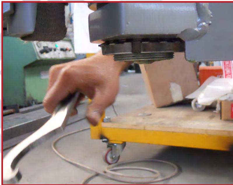
**30.** Insert the safety washer and screw the ring nut on the pin.
