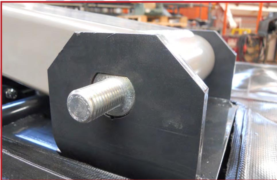
**64.** Position it close to the protection's assembly, remove and re insert the pin of the guards like shown in the picture.
