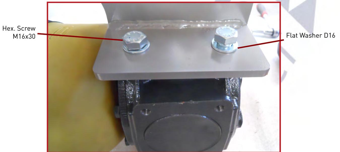
**45.** Screw it at the 3rd point and tighten the locking screws.
