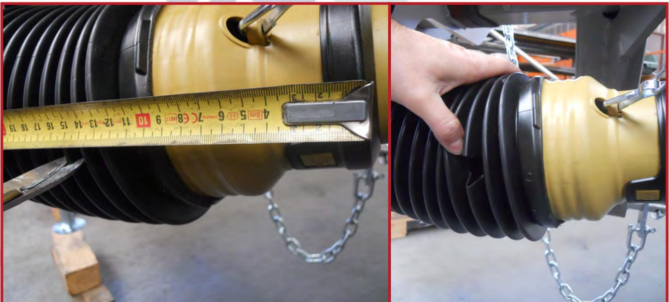
**76.** Make a hole on the 3° ring of the rubber bellows like shown in the picture.
