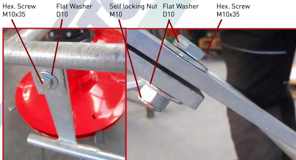
10. Insert in all the holes screws, washers and nuts.
