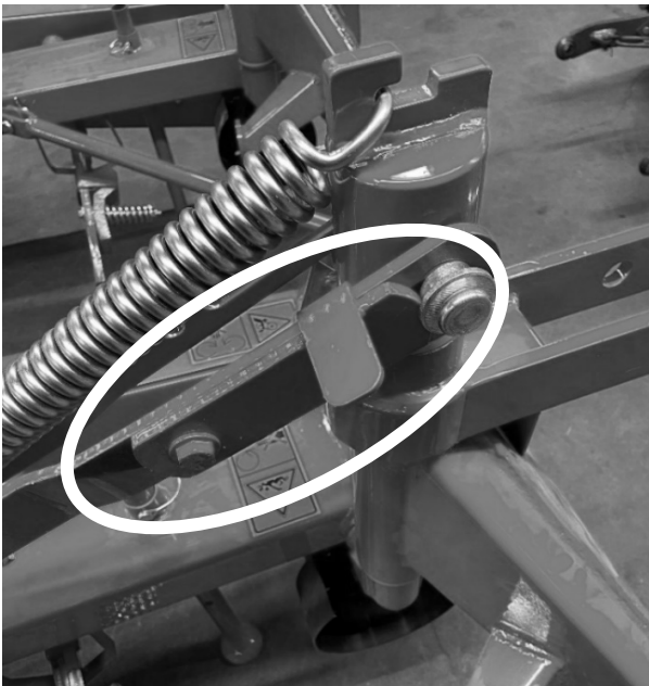
Figure 2 – Transport lock, shown in the locked position
