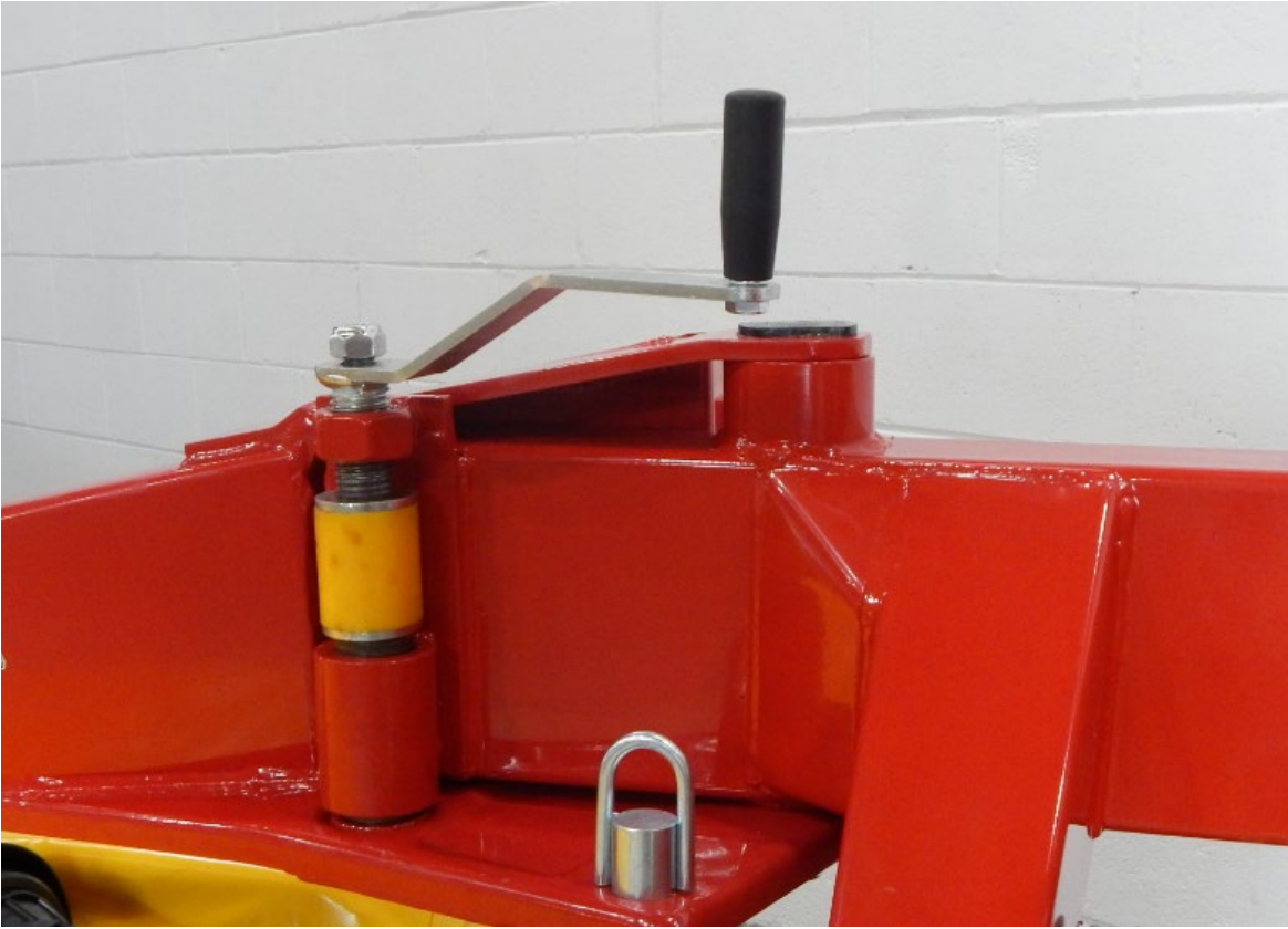
Figure 3 - Safety release lever installation
