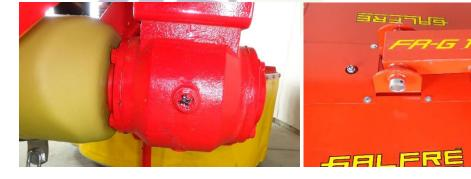
Verify the level of the oil in the right angle gearbox on the three point hitch. The level should be half way up and filled to the level of the plug on the side. Refer to the owner's manual for oil type. Although units are shipped with oil, it is always a good idea to check them one last time before first use.
