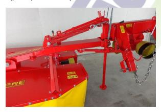
Figure 34 lift the three point assembly up and install the jack stand
