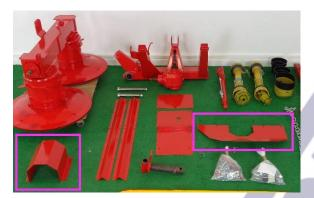
Figure 22 PTO shields
