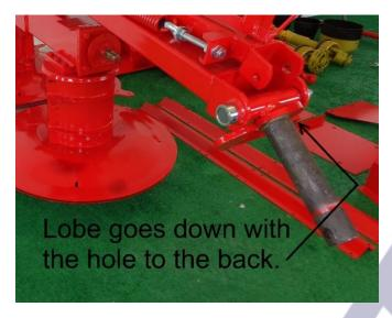
Figure 13 install pin with hole to back
