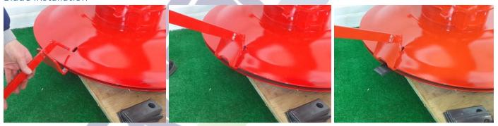
Figure 14 installing blades with the blade change tool
