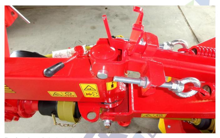
Figure 2 rear of mower showing pivot pin orientation
