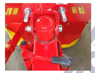
Figure 27 top cap and spring arm bolted in place on a model 170 mower
