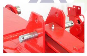
Figure 9 long pin goes through as shown
