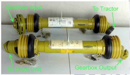
Figure 35 driveline identification and connection guide
