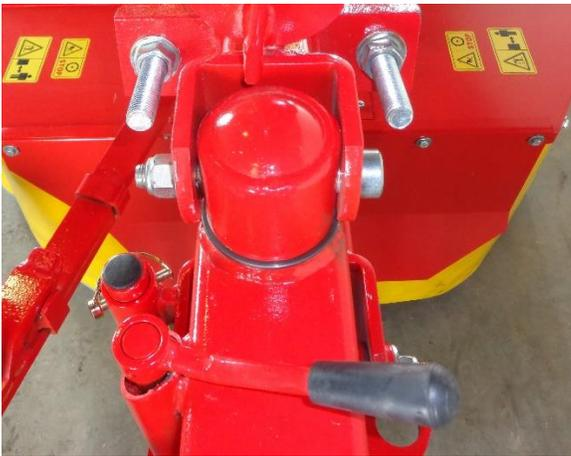
Figure 27 top cap and spring arm bolted in place on a model 170 mower
