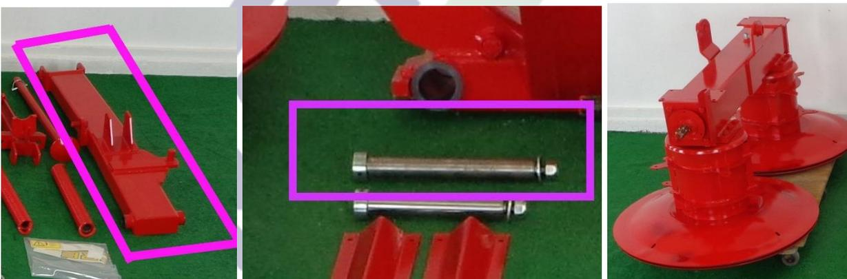
Figure 6 parts to connect arm to drum
