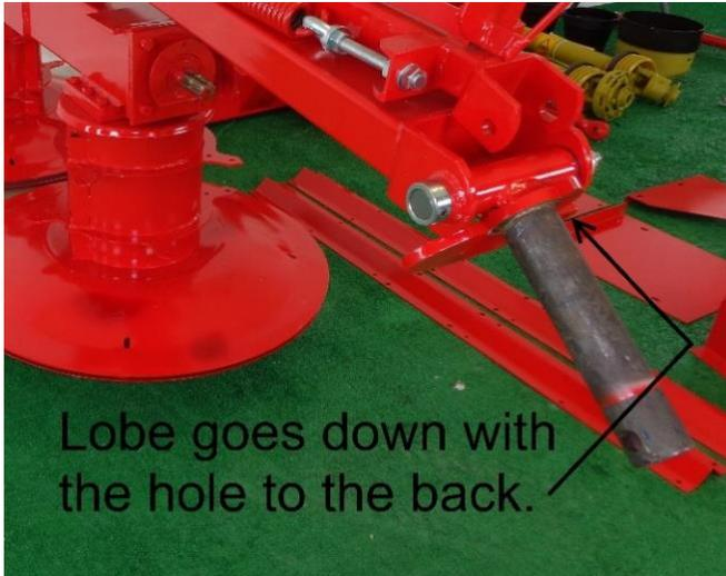
Figure 13 install pin with hole to back
