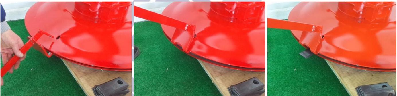
Figure 14 installing blades with the blade change tool
