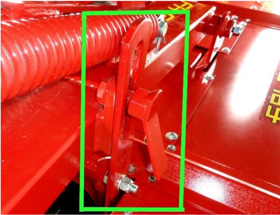
Figure 33 pivot restrictor plate shown installed but loosened 2 turns for mow position
