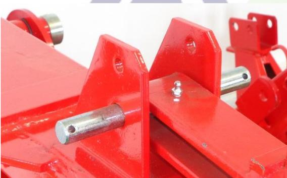
Figure 9 long pin goes through as shown
