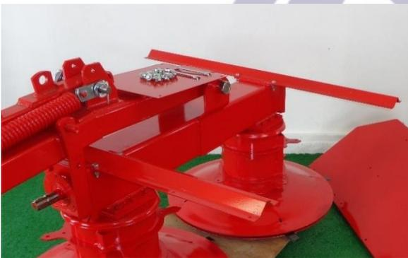
Figure 17 guard holders shown installed on both ends of the 190 drum unit
