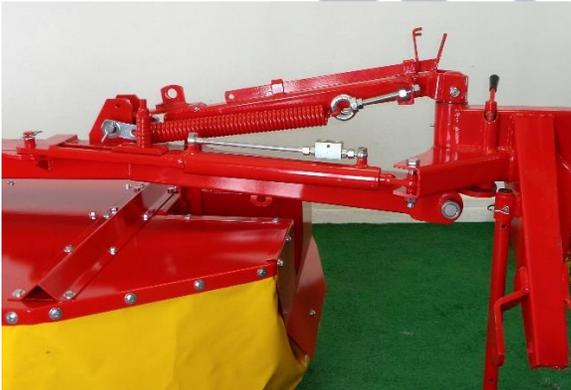
Figure 28 hydraulic cylinder for transport / mow positioning on a 190 mower
