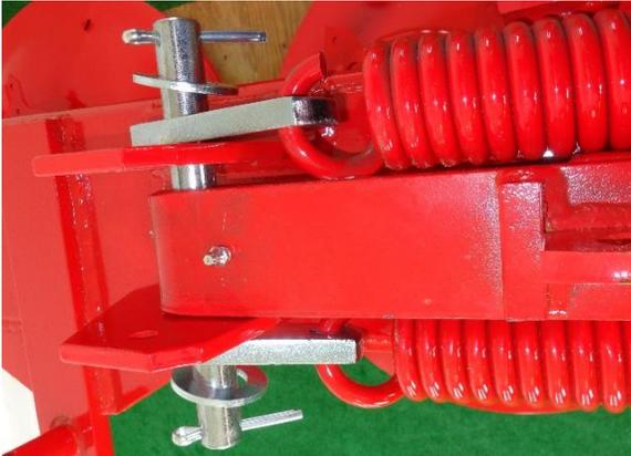
Figure 10 spring attachment hardware shown with springs
