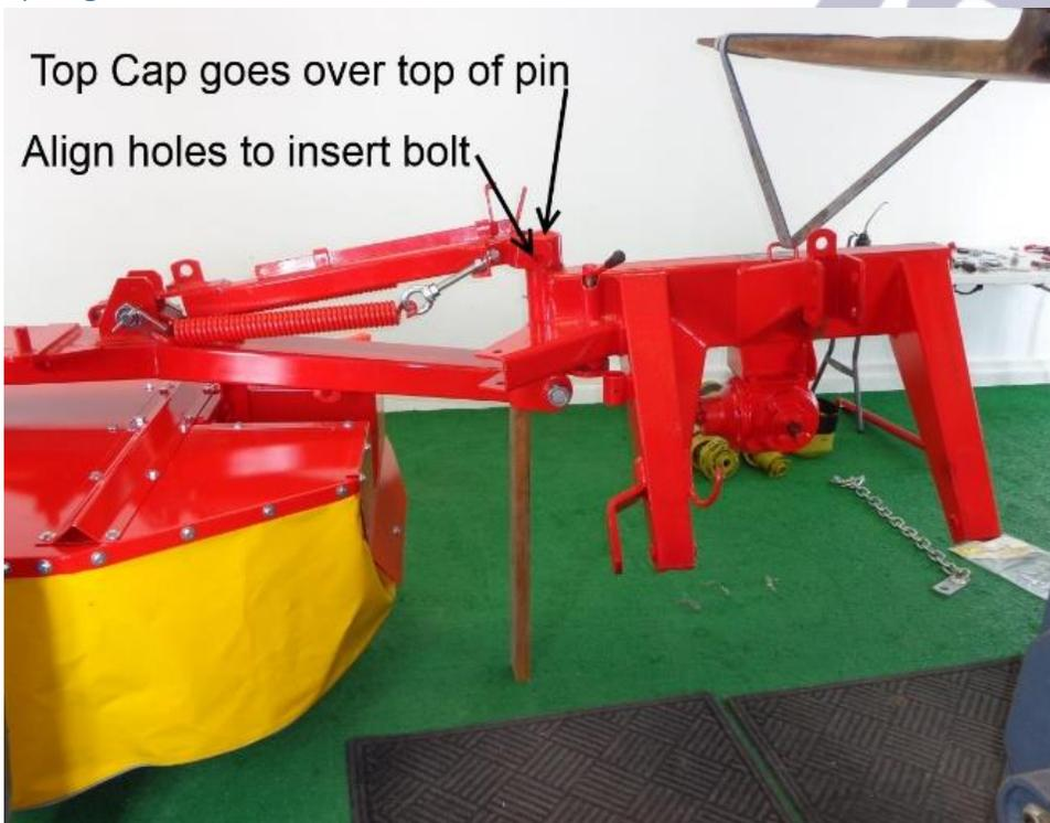
Figure 25 hang 3 point hitch and connect to mower
