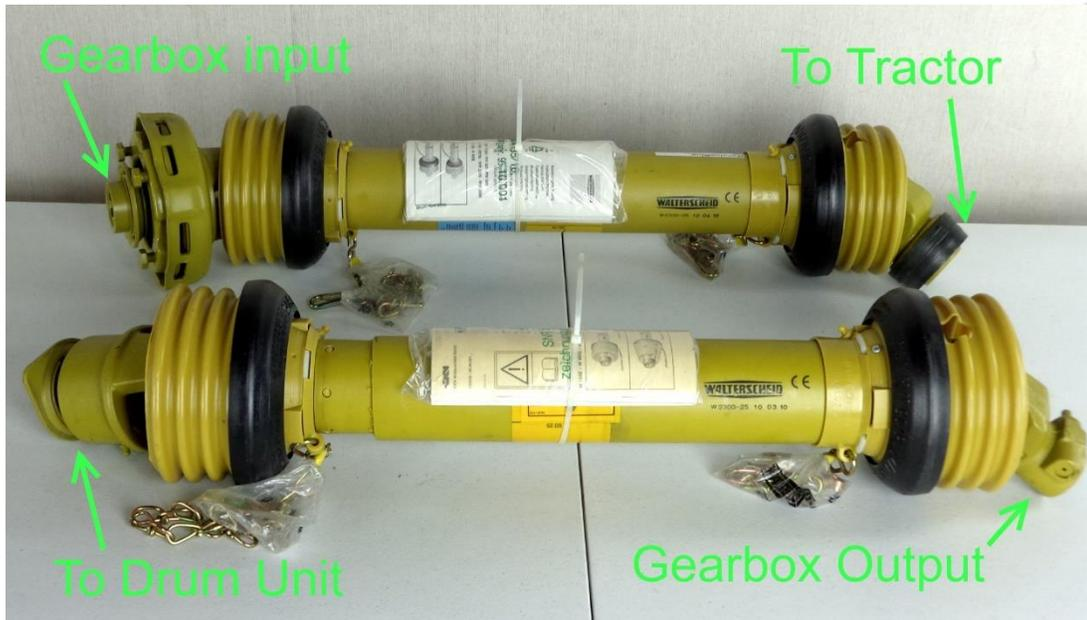
Figure 35 driveline identification and connection guide
