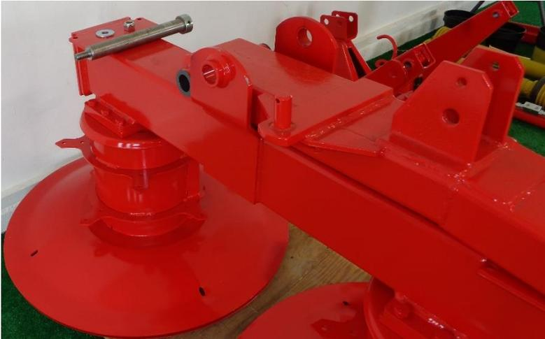
Figure 7 model 190 drum assembly with arm before attachment
