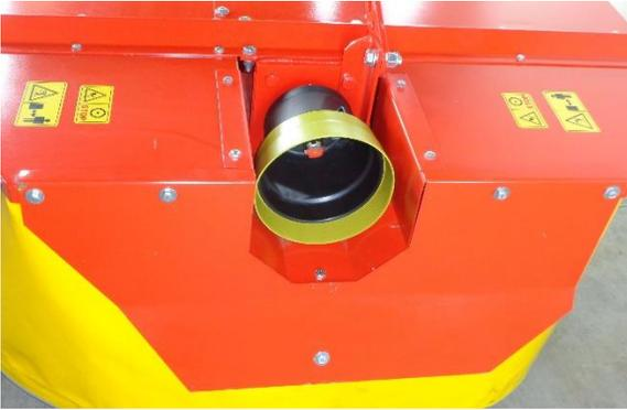
Figure 24 shields installed as well as PTO guard on a 170 drum unit
