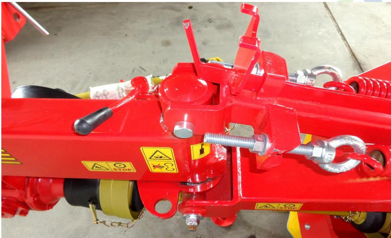
Figure 2 rear of mower showing pivot pin orientation
