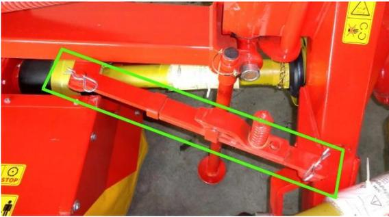
Figure 29 manual swing model 170 break away protection arm in mow position
