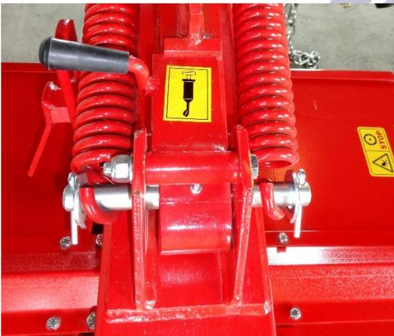
Figure 31 spring arm transport lock shown installed and in transport position on a model 170 mower
