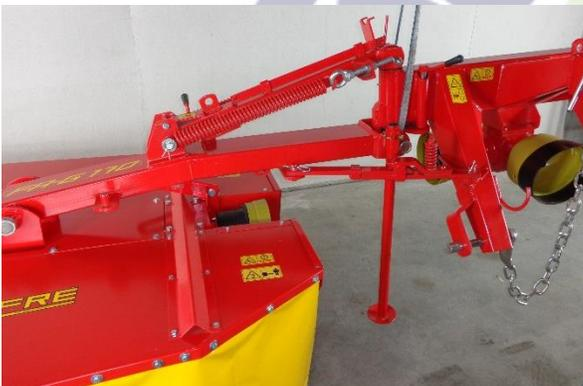
Figure 34 lift the three point assembly up and install the jack stand
