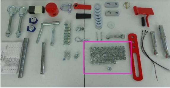
Figure 18 set of 48 nuts and bolts are for guards and shield plates on a 190 mower
