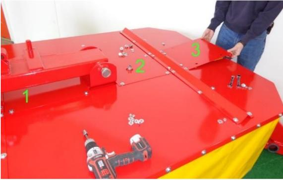
Figure 21 shield plates shown located on top of guards on a 190
