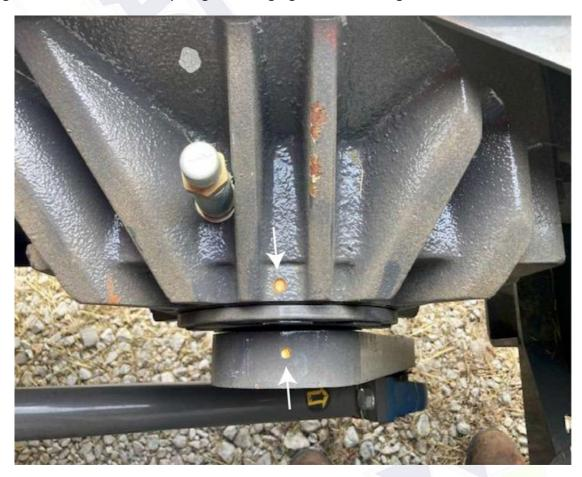
2. With the crank arm in this position, the timing dots on the fork drive sprockets should align with the dots on the frame, as seen in the picture below.
