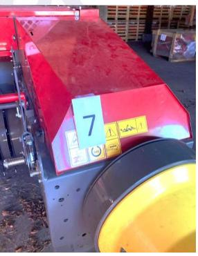
Remove the knob that retains shield 7 and secure it in the open position with the support stand.
