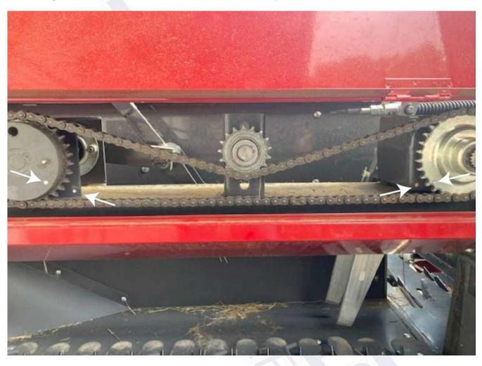
3. Check that the timing dots on the bell gear ref. 3 and on the frame are aligned. See below and also Fig. 7.7 in the Sitrex Manual.
