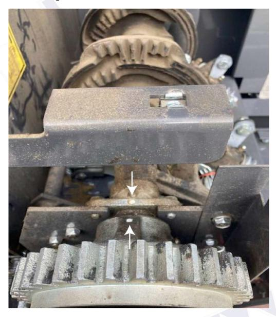
If all components are found to be in time, the timing process is not required. If any components are found to be out of time, proceed with the timing process. Prior to beginning the timing process, remove all hay from the bale chamber.
