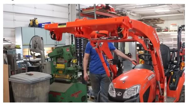
Unthread the stand release foot bolt (3/8" wrench) until it contacts the stand release foot and then unthread an additional turn.
