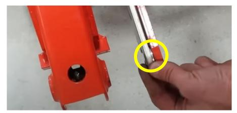
9. Clean old grease off of pins and mounting holes.
