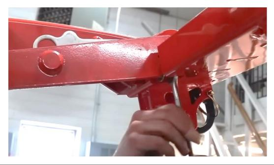
22. Tighten the first jam nut against the washer (9/16" wrench) and then tighten the second against the first.
