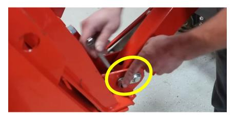
4. GEN 1: Remove cotter pins (reused later) from outside of loader arm pins.
