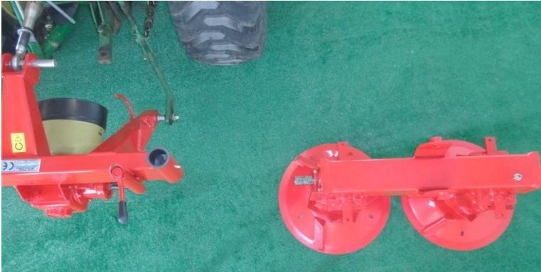
Figure 13 move the drum unit over to the three point hitch assembly like this
