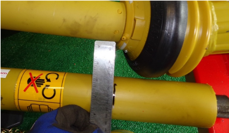
Figure 39 mark overlap length
