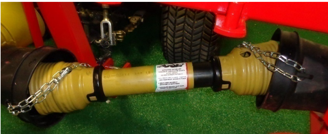
Figure 29 guard chains attached
