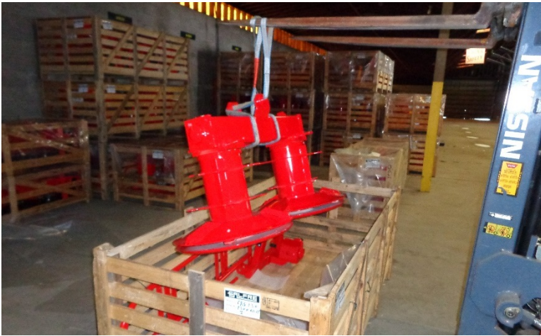
If no lift is available, the crate will need to be cut open for easier access. Remove the smaller parts, then slide the drum unit out of the crate onto the ground. The drum mower bottom skids drag across the ground during use, so it is alright to drag them to the location that you plan to use for assembly.
