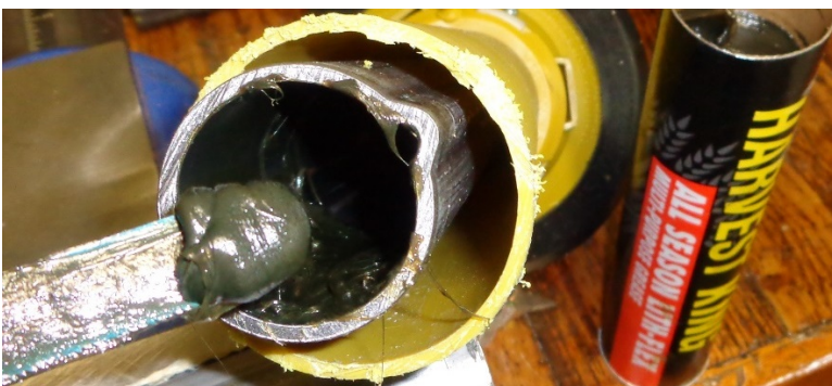
Figure 48 spread grease inside outer shaft
