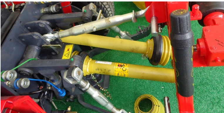
Figure 38 PTOs installed to mark overlap
