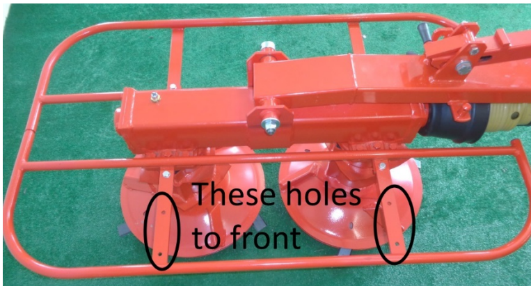
Figure 33 front guard has 6 holes
