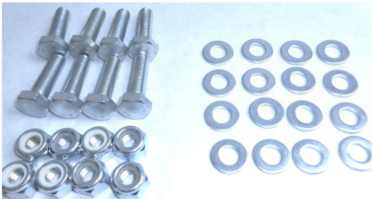
Figure 34 eight sets of fasteners used for attaching guard frame
