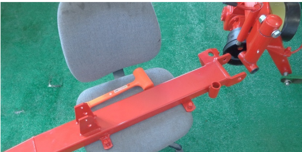
Figure 18 align holes in arm to swivel tee
