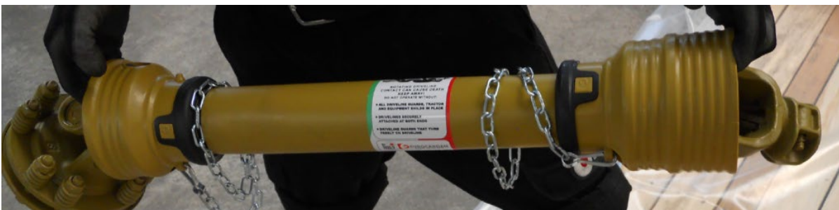
Figure 30 shaft with slip clutch end
