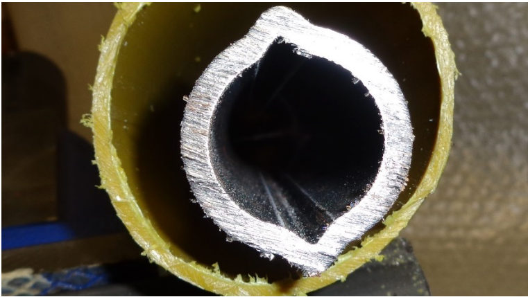
Figure 46 burrs and shavings must be removed
