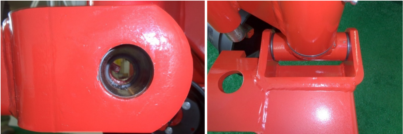
Figure 19 holes aligned to allow pin to pass
