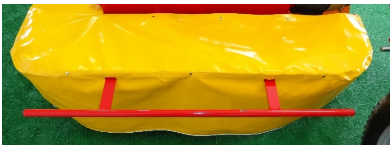
Figure 35 curtain installed with 2 holes for toe guard facing forward
