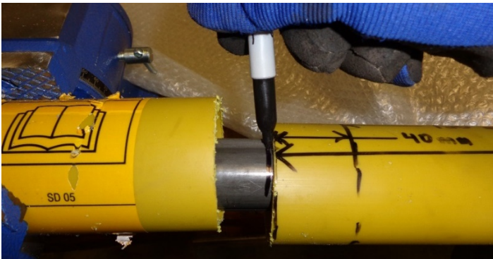
Figure 43 use tube to mark the cut length to steel shaft
