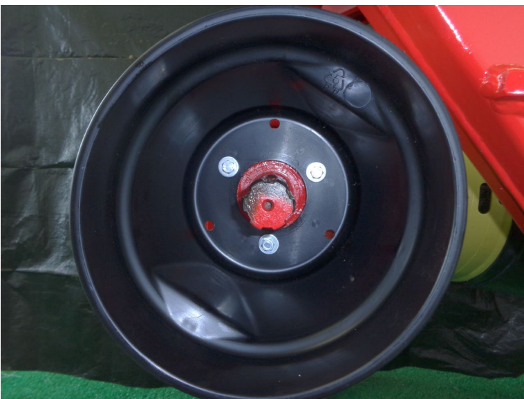
Figure 7 the third guard is installed on the remaining location on the 90 degree gearbox
