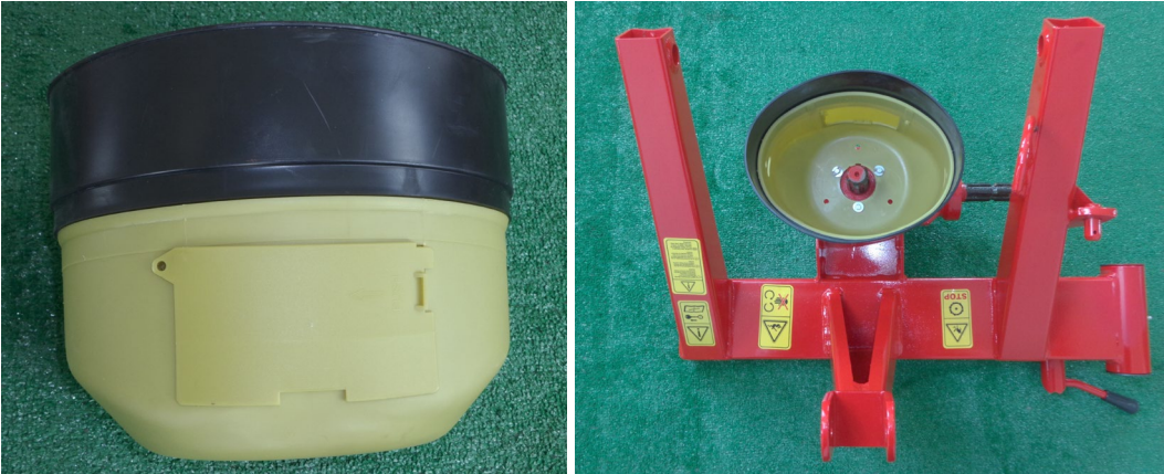
Figure 5 the large guard installs on the gearbox facing the tractor
