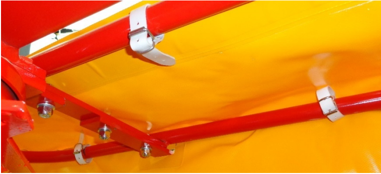
Figure 36 curtain straps secure to the guard frame
