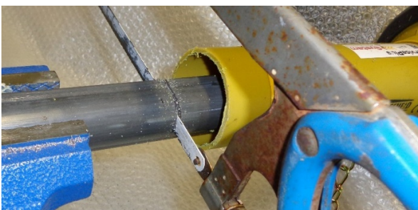
Figure 45 clamp on the part of the shaft that is being cut off, then cut
