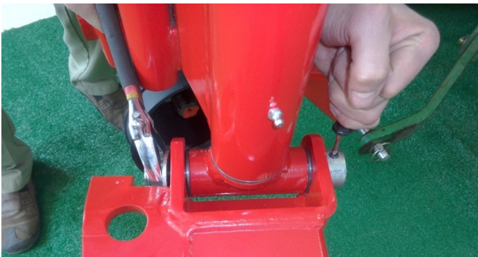
Figure 20 pin through and nut started
