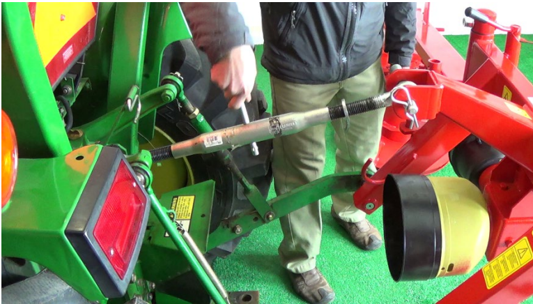
Figure 10 level the 3 point hitch unit with the top link
