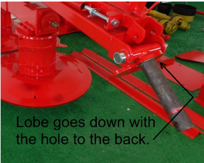
Figure 13 install pin with hole to back
