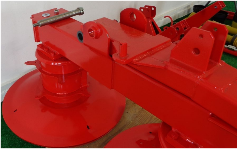
Figure 7 model 190 drum assembly with arm before attachment
