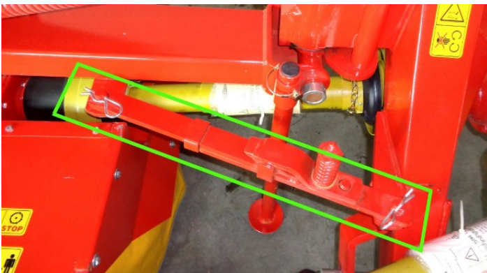
Figure 28 breakaway protection arm in mow position
