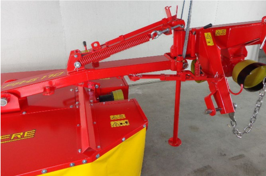
Figure 33 lift the three point assembly up and install the jack stand
