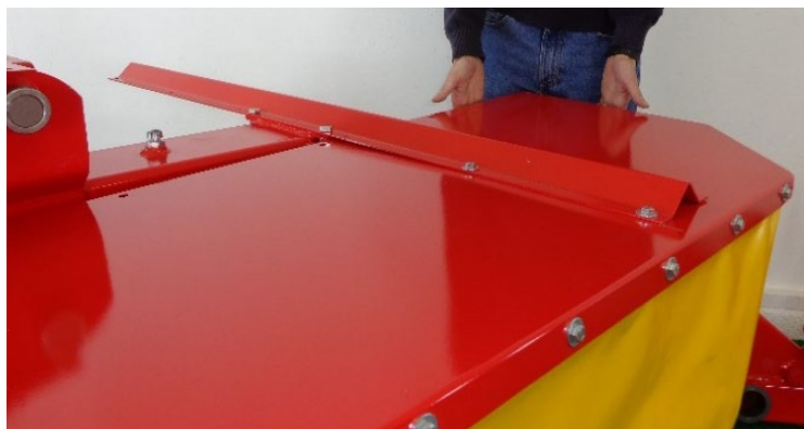
Figure 19 guards hang from the guard holders and are secured with hardware shown
