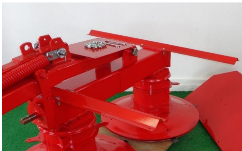
Figure 17 guard holders shown installed on both ends of the drum unit
