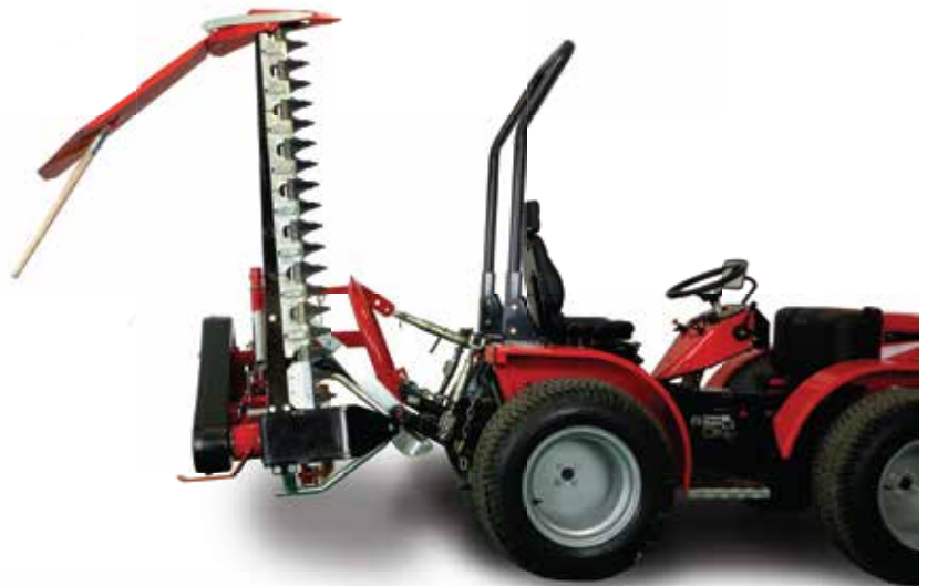
Mechanical lift system requires no tractor hydraulics
