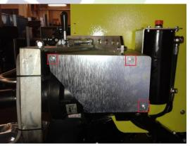
Remove the side panel shown in picture. The control box connector has to be plugged in here.
