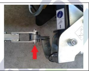
Couple the drawbar to its supporting element as shown in picture. Fasten the nut well.
