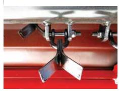
Multiple mounting options allow for varied offset and better fit on different sized tractors.
