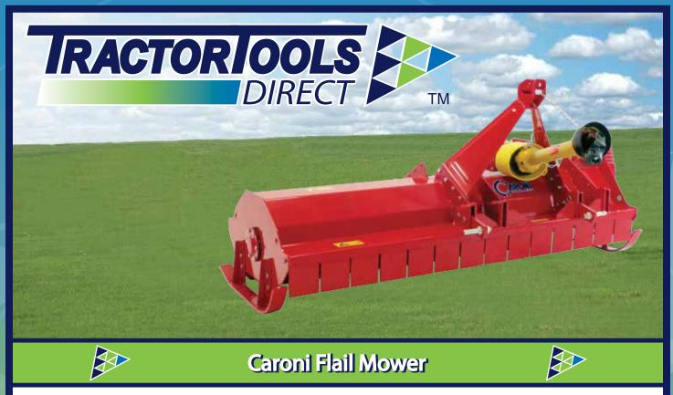
The Caroni TM series of flail mowers, suitable for tractors ranging from 20 to 60 HP, are ideal machines for maintaining field edges, trails, pastures, and clearing overgrown areas and brush.
